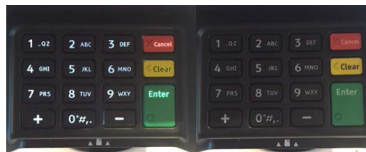
Left: backlight visible when keypad is shielded. Right: no backlight visible
